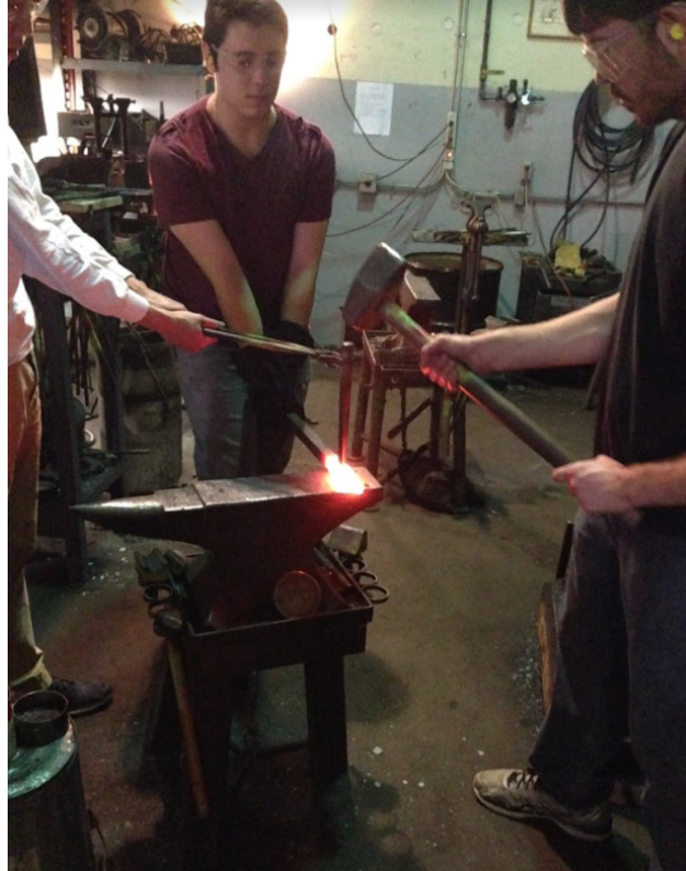
Figure A.3: Three person team punching the hole where the handle would be inserted. After creating the spike shape, we would drive a tapered steel rod into the middle of the bar. We placed the bar over the hole located in the rear of the anvil so when the steel rod penetrated the bar, the rod could create a larger hole. Every three hits, the tapered rod would be removed, cooled in water, and covered in graphite as a lubricant. If these three steps were not performed, the tapered steel rod would merge with the bar that we were trying to forge.
