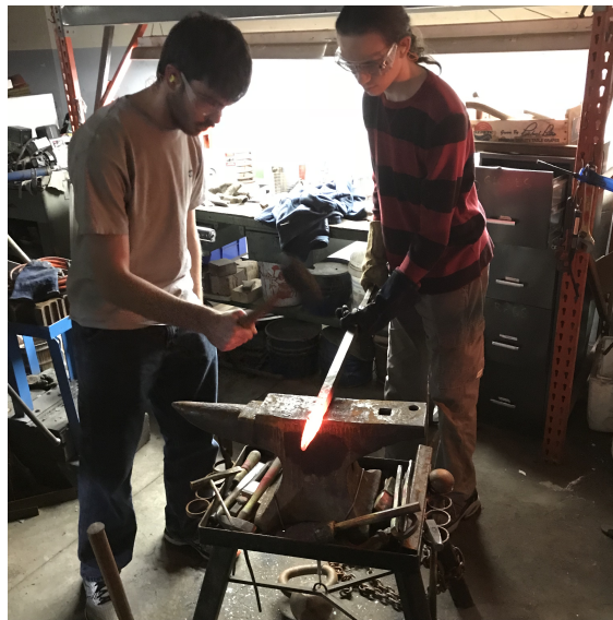
Figure A.2: Shaping the end of the steel bar to form a spike.
