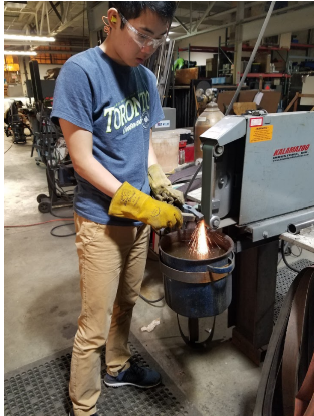
Figure A.5: Smoothing and polishing the shaped head. By using a motorized sandpaper wheel, we smoothed and polished any rough edges present on the hammerhead. Because of the heat created by the friction, the hammerhead was cooled every minute in the bucket of water located under the sandpaper in the figure.
