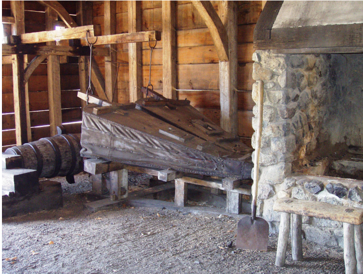
Figure 2.8: An interior view of a reconstructed forge with bellows operated by water power, located at the Saugus Iron Mill in Massachusetts. ( Saugus Iron Mill - forge with bellows , 2006)
