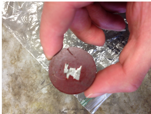
Figure 5.1: A sample square of metal immediately after being pressed into a mount.
