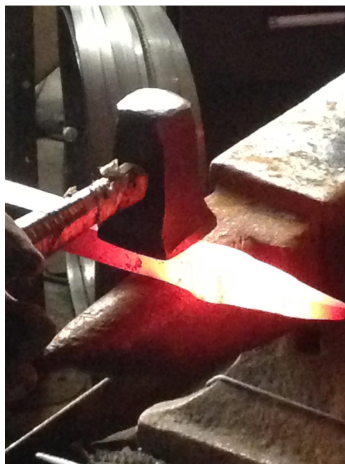
Figure 4.5: Manually forming the grooves while shaping the face of the warhammer.
