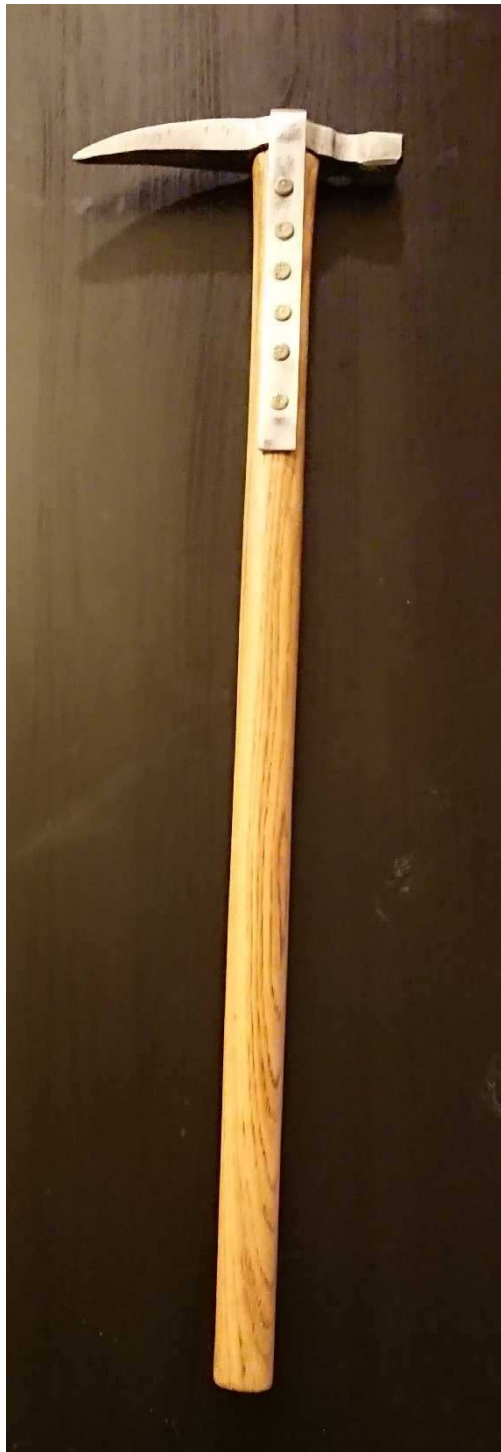
Figure A.9: Finished war hammer after attaching the langlets and applying the polyurethane coating.
