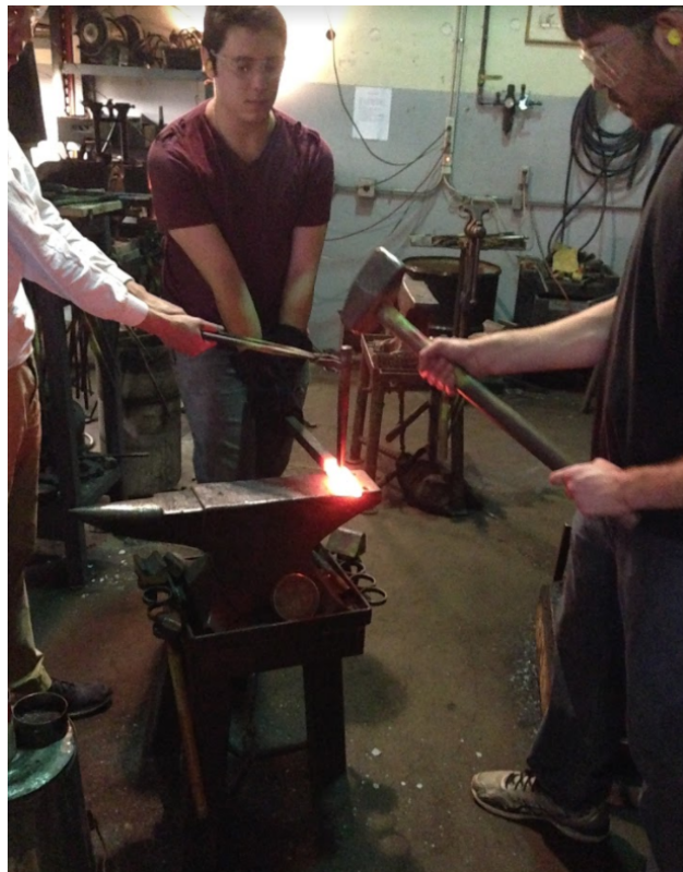
Figure 4.4: Three person team punching the hole where the handle would be inserted.
