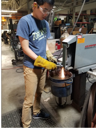
Figure 4.7: Deburring of the piece using belt sanders.
