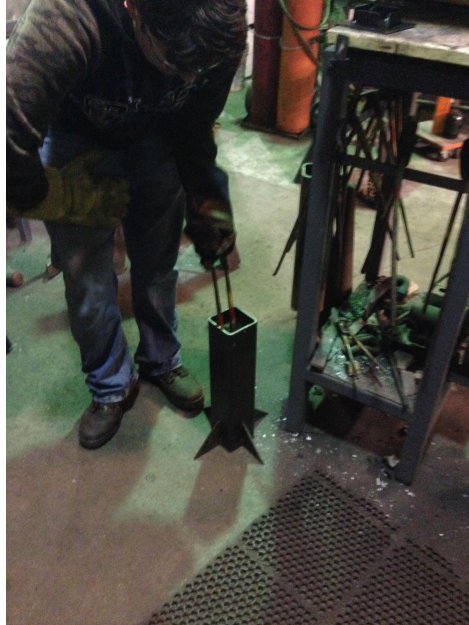
Figure A.6: Quenching the hammerhead in oil after heating it past the Curie point. We repeated the previous processes above for our final hammerhead. This was done because our first hammerhead was a prototype where we would familiarize ourselves with the forging methods used. After repeated these steps, we heat treated our final hammerhead by quenching it in oil. This would reduce the risk of it cracking compared to water because the hammerhead would not cool as quickly.
