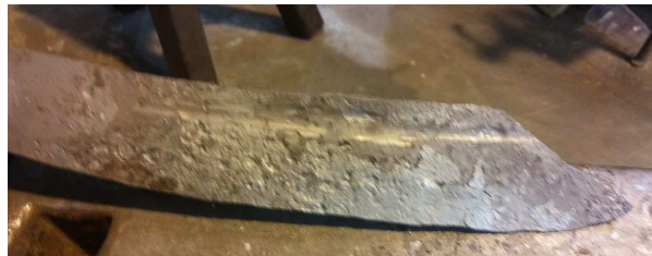
Figure 28. Close up of the edge of the larger dao at the end of Day 5 of forging.
