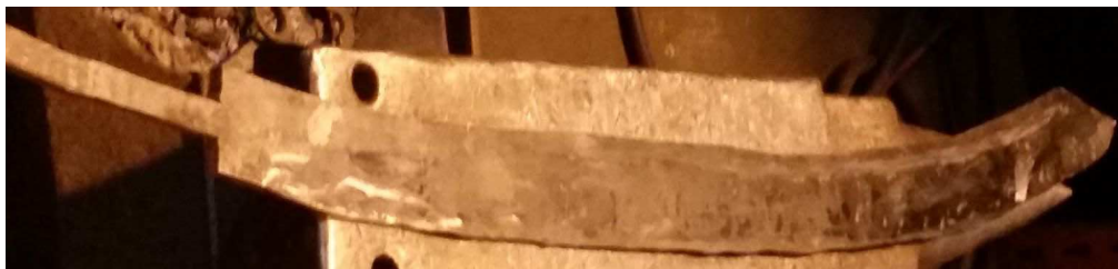
Figure 34. The larger dao after the tenth day of forging.
