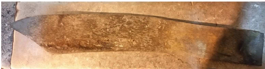
Figure 24. The practice dao after quenching.
