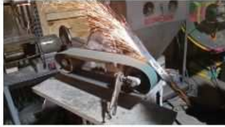
Figure 4 - Grinding the Dao.
