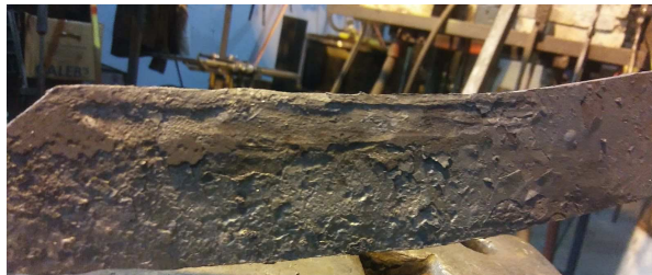
Figure 21. Close up of the blood groove on the smaller practice dao at the end of Day 5 of forging.
