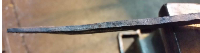
Figure 27. Close up of the thickness of the tip of the full-sized actual dao at the end of Day 4 of forging.
