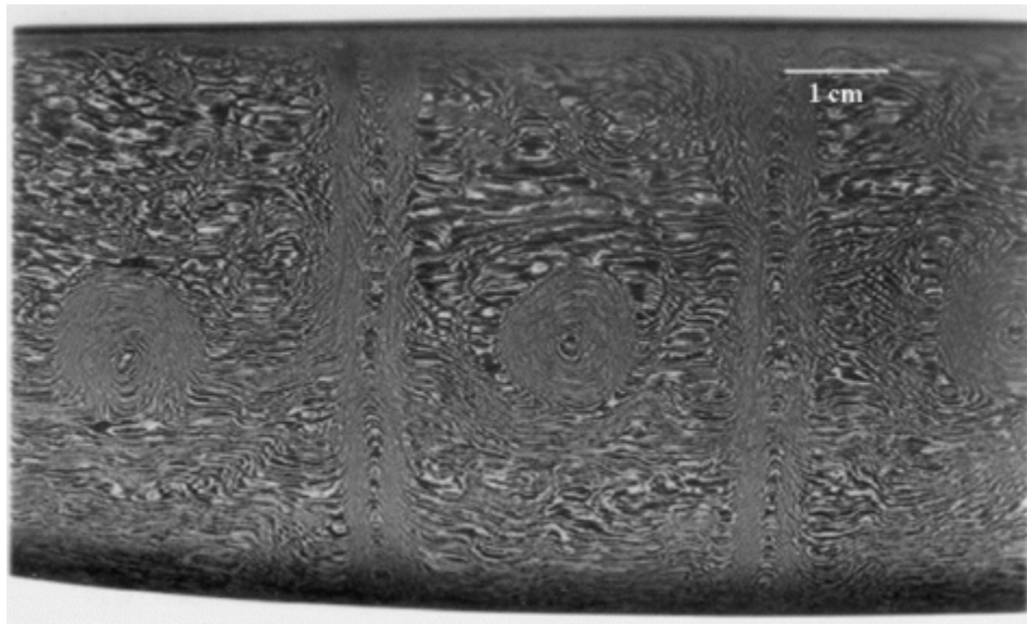
FIGURE 7. CARBIDE PATTERNS IN DAMASCUS STEEL.
