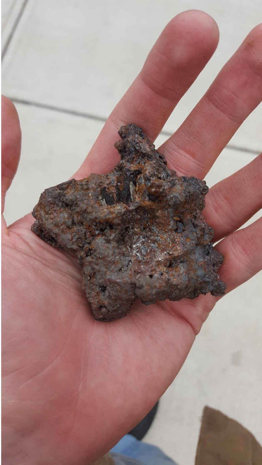
FIGURE 14. PART OF THE COOLED BLOOM.
