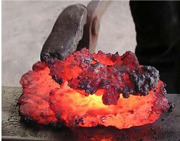
FIGURE 2. AN EXAMPLE OF AN IRON BLOOM.
