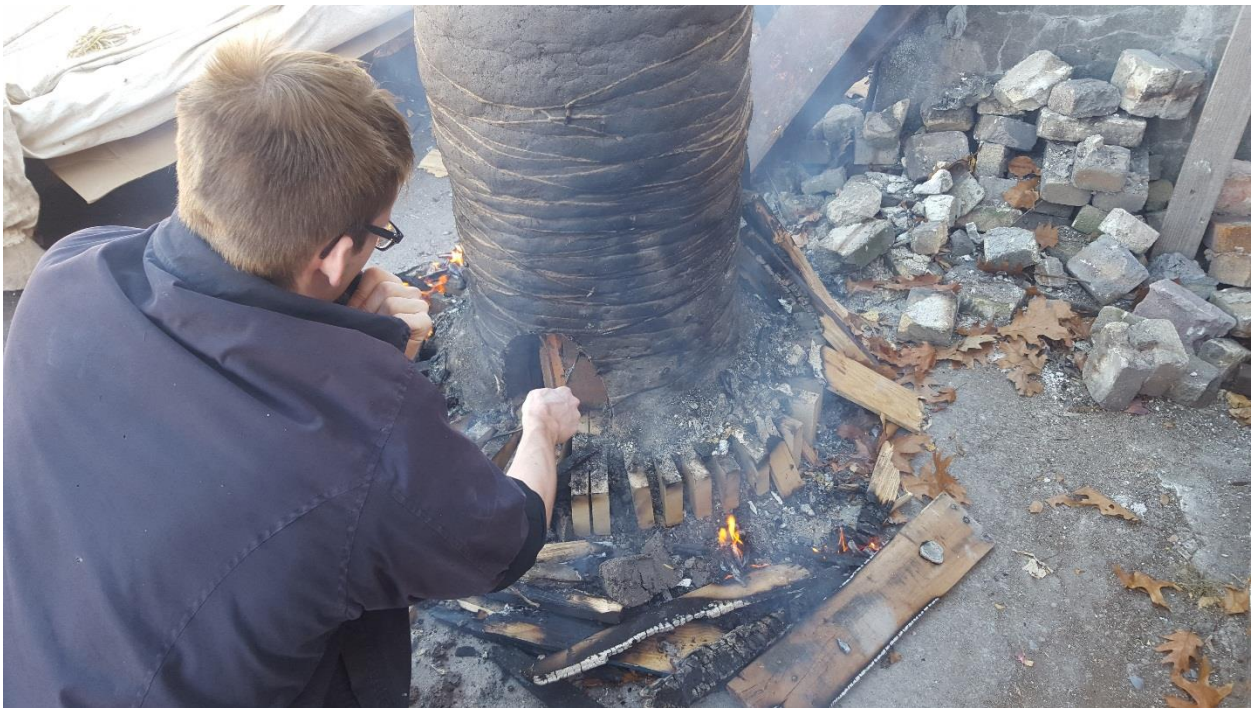
FIGURE 8. CUTTING THE TAP ARCH
