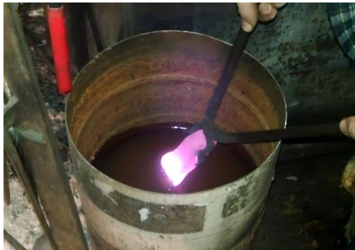
Figure 8 - Quenching the Axe Blade and Barb.
