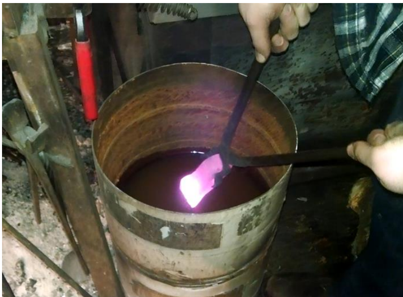
Figure 38. Quenching the blade.
