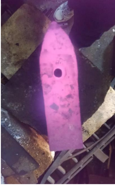
Figure 34. Punched hole, slowly expanding.
