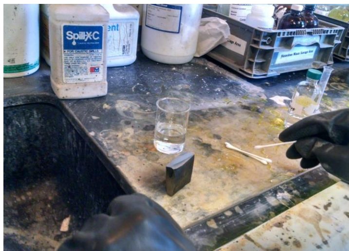
Figure 41. Testing the Nital solution.
