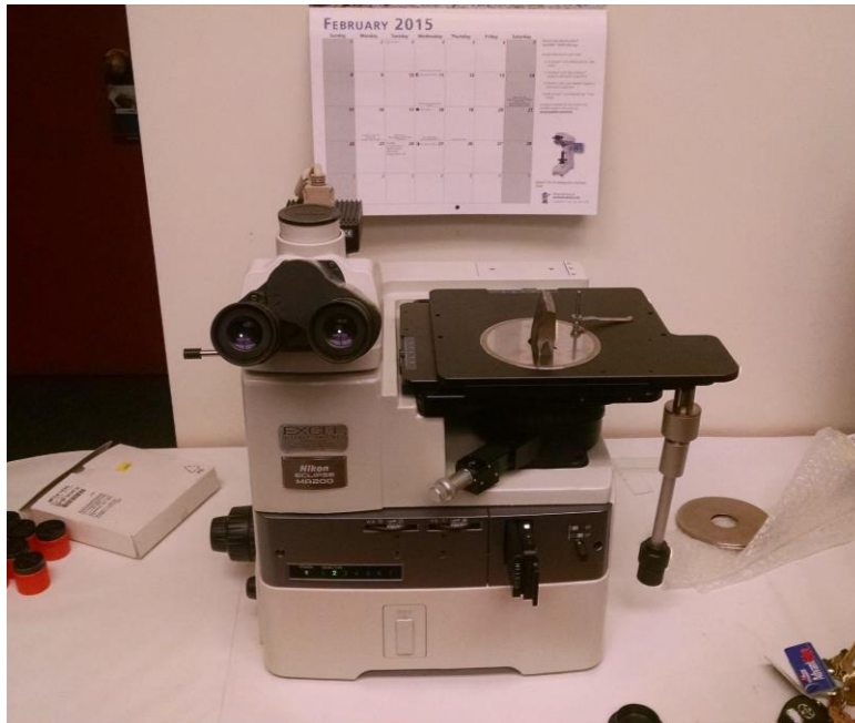
Figure 42. Optical microscope used for microstructure analysis.
