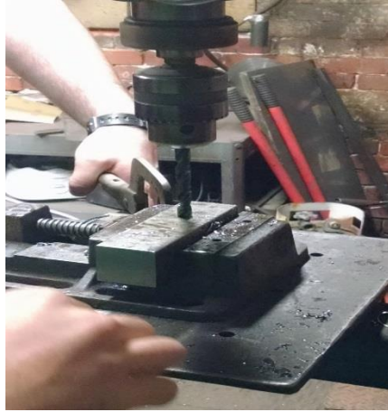
Figure 2 - Drilling of Pilot Hole.
