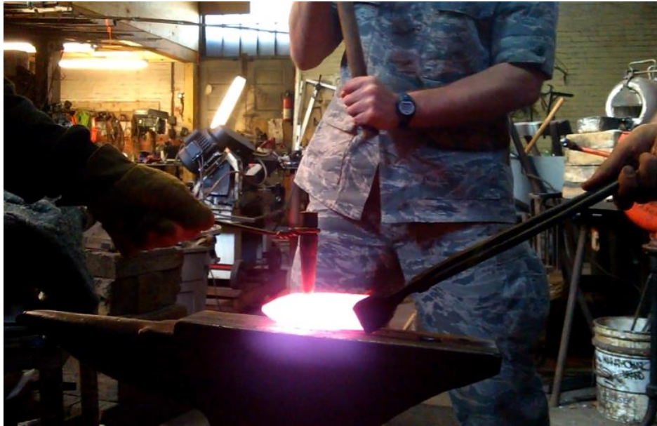
Figure 33. Hammering punch to create handle hole.
