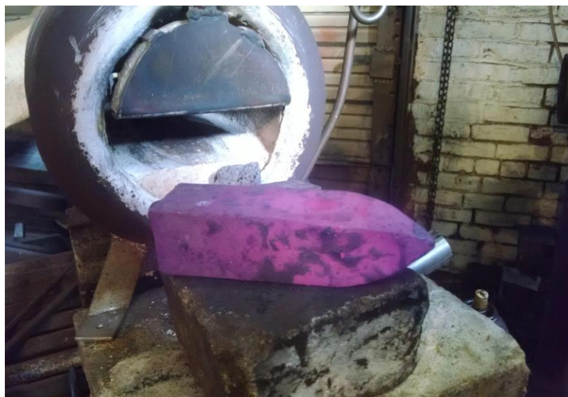
Figure 32. The axe head cooling after drawing out the point.
