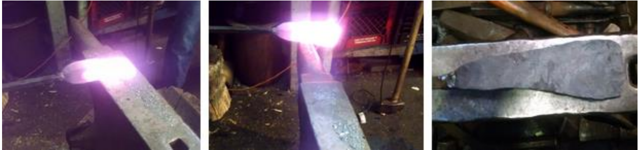
Figure 5 - Drawing Out the Axe Blade.
