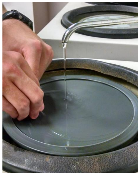
Figure 40. Samples being polished.
