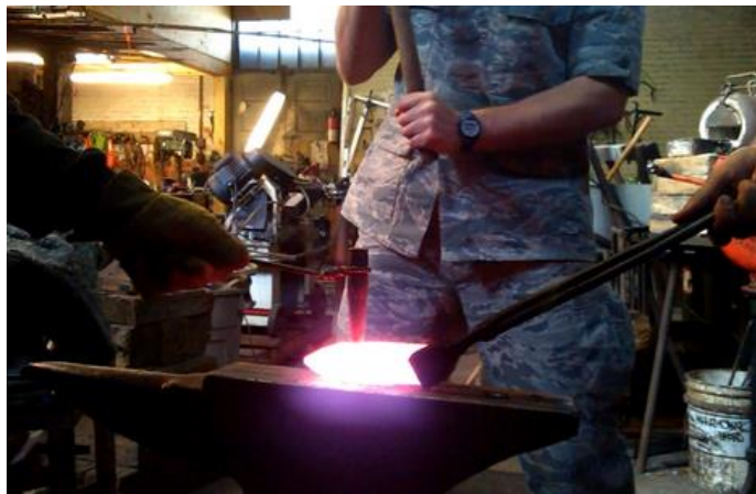
Figure 4 - Punching an Axe Handle Hole.
