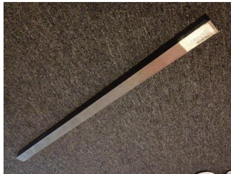
Figure 1 - 1.5 in by 1.5 in by 36 in 1045 Steel stock.
