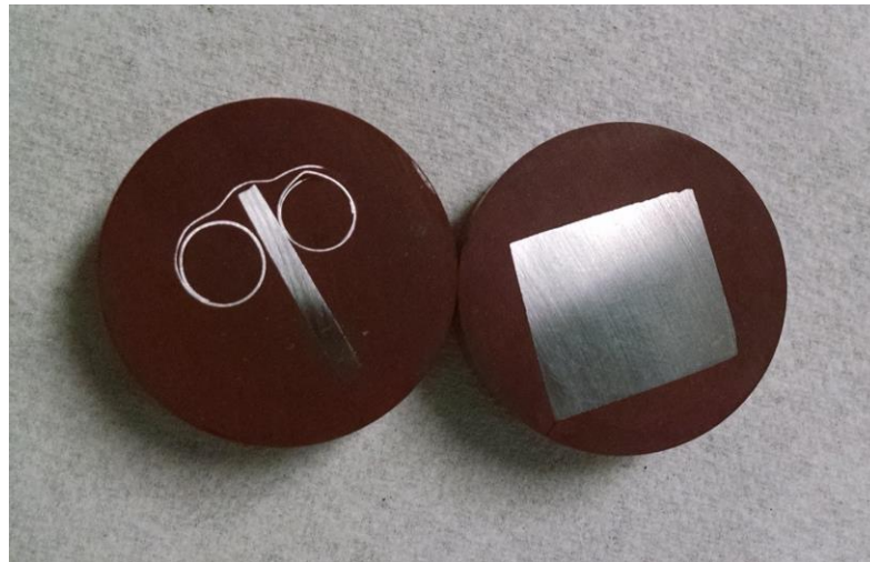
Figure 39. Mounted samples ready for polishing.
