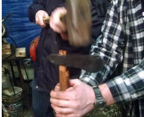
Figure 7 - Attaching the Axe Handle.
