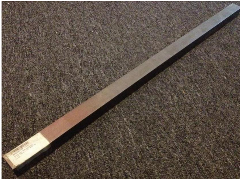
Figure 27. Our 1045 Steel rod before metalworking.
