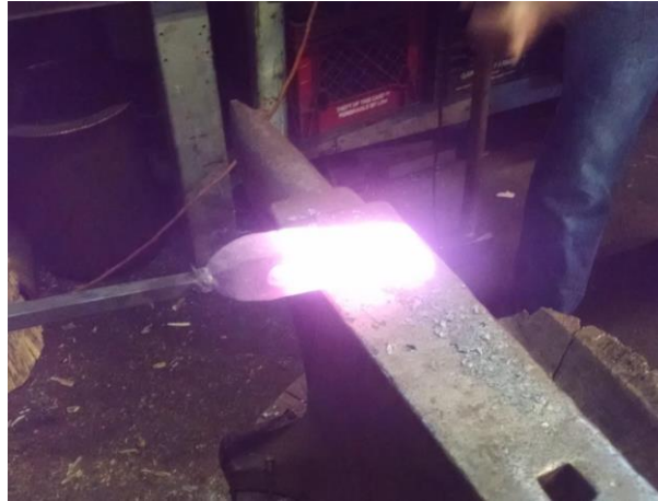
Figure 35. Wedge hammer to stretch metal horizontally.
