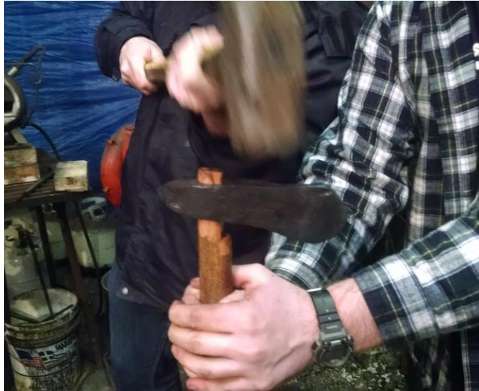
Figure 37. Securing axe head to handle.
