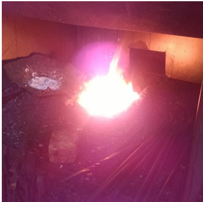
Figure 31. The forced air coal forged, located in Ferromorphics main shop.
