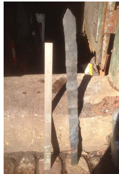
Figure 21: Initial bar vs. shaped Gladius.
