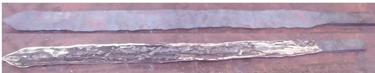
Figure 22: Comparison of worked (top) vs. surface-finished (bottom) blade.
