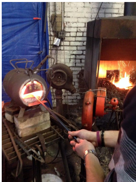
Figure 22: Heating the metal in the propane forge
