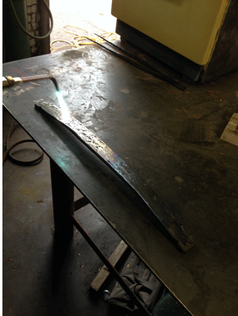
Figure 27: Heating the metal with the torch
