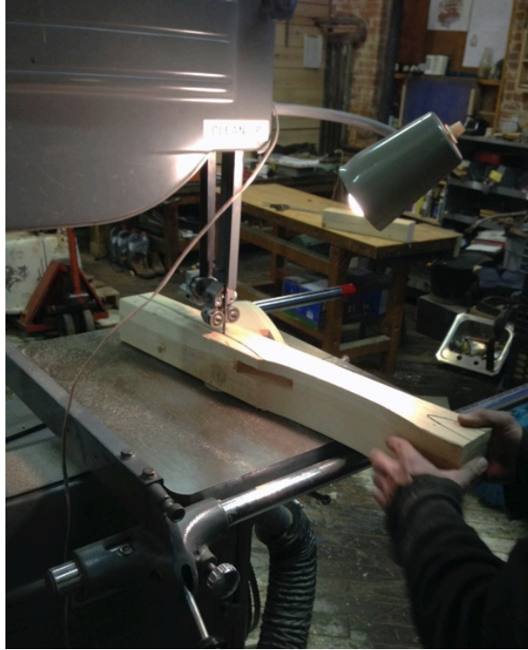
Figure 37: Cutting the stock
