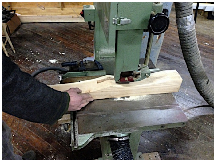
Figure 36: Cutting the excess of the stock
