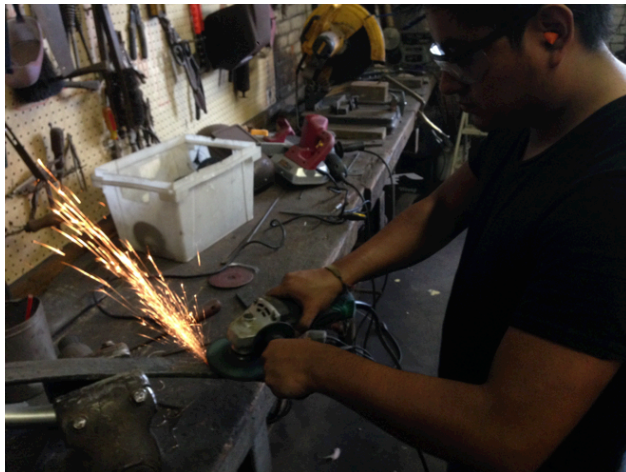
Figure 26: Grinding the metal
