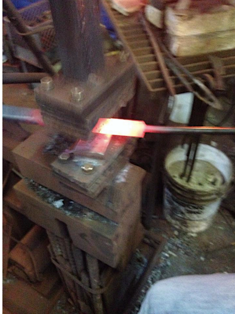
Figure 23: Hammering the metal in the power hammer
