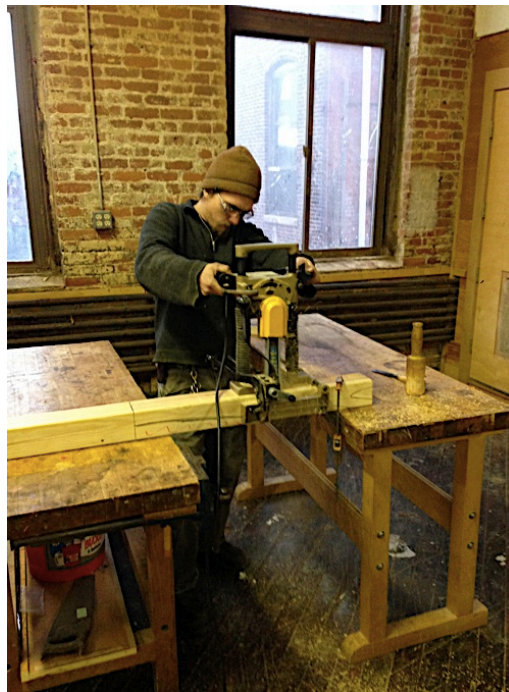
Figure 33: Drilling the trigger hole
