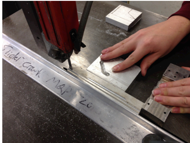
Figure 30: Cutting the handle
