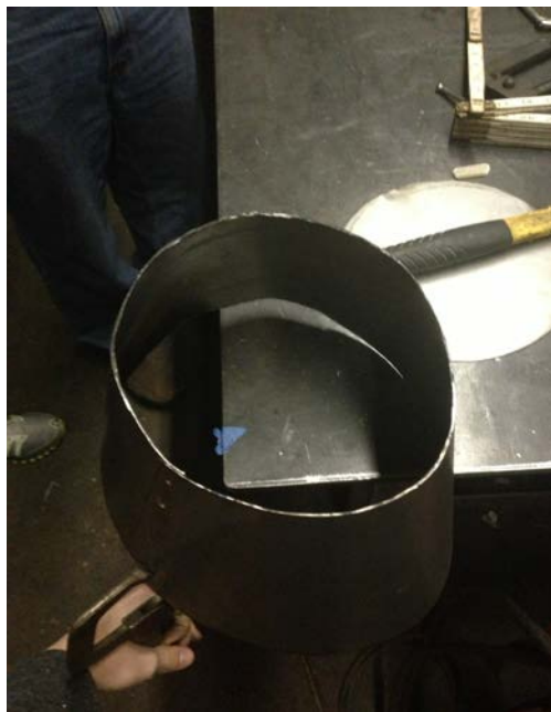
Figure 47: Top frustum after riveting.
