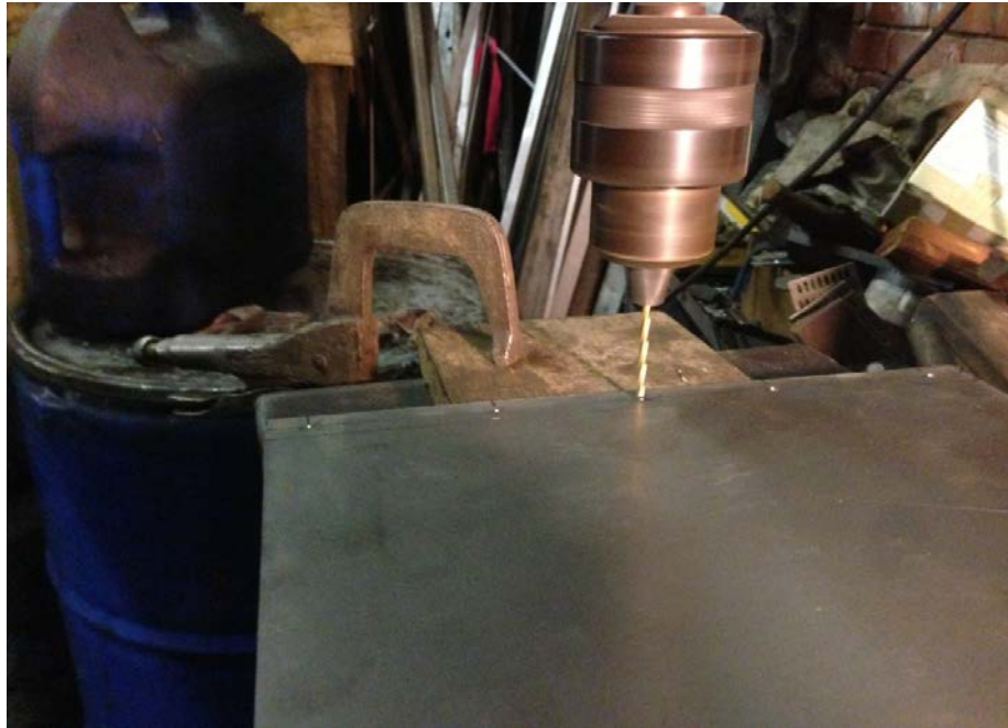
Figure 40: Using a drill press to make holes in the metal.
