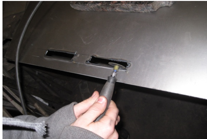
Figure 31: Using a dremel to shape the edges of the eye slits.
