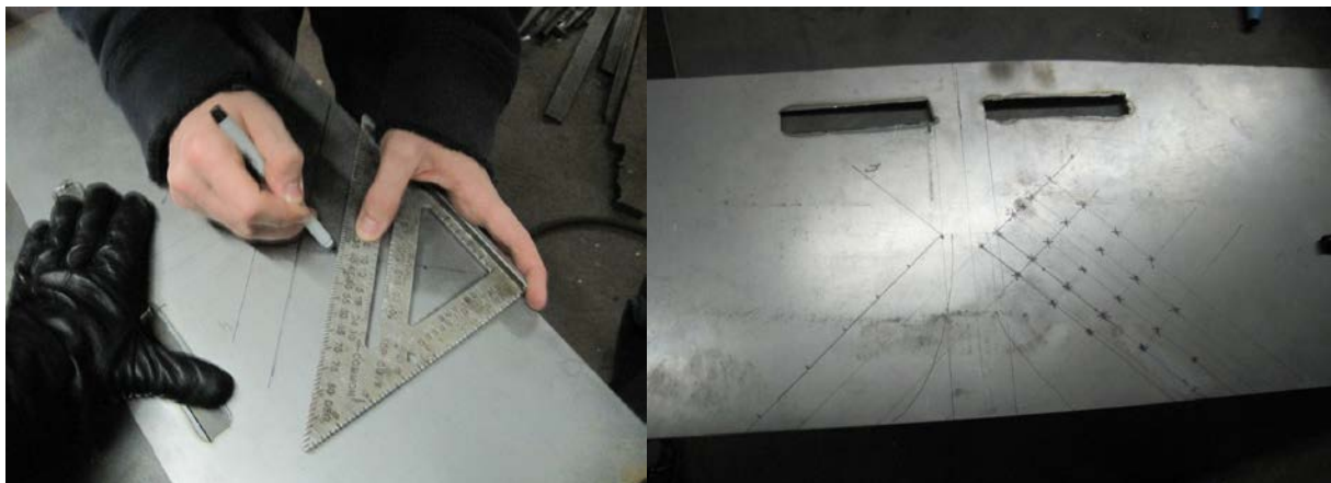
Figure 32: Drawing the breathing hole pattern onto the steel.
