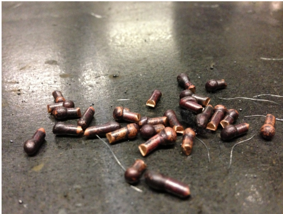
Figure 38: Copper rivets created from melting copper wire.
