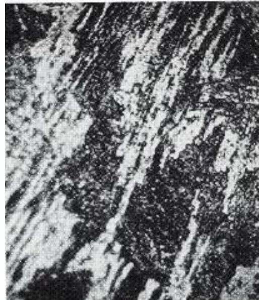
Figure 10: Photomicrograph of steel with bainite (Williams, A).
