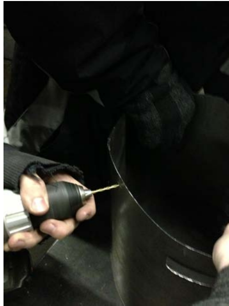
Figure 48: Drilling holes for the rivets and tabs on the bottom piece.
