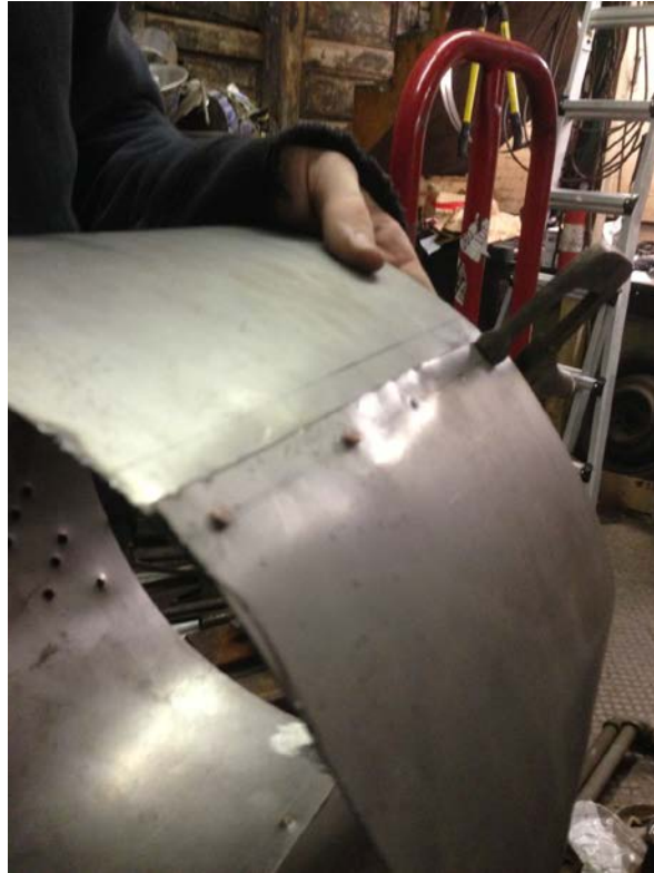
Figure 44: Riveting the bottom part.
