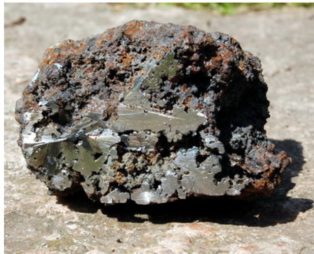
Figure 4: Cut away of an iron bloom (Web: "Making Iron").
