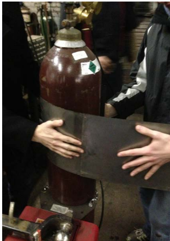
Figure 43: Bending the bottom piece around a curved surface to form a cylinder.
