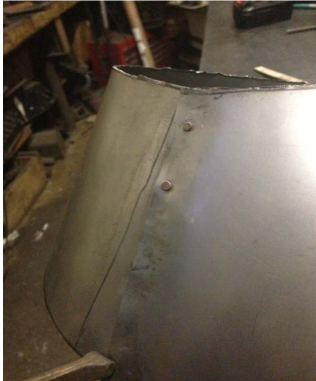
Figure 46: Riveting the frustum together, using a clamp to apply pressure.
