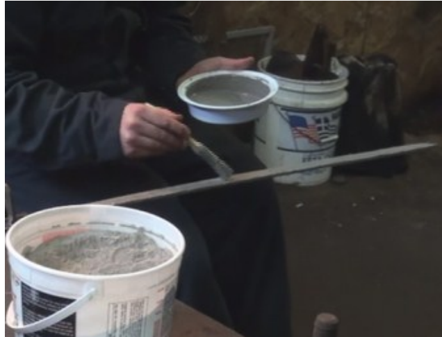
Figure 38: Applying Refraction Clay to the Blade Before Quenching.
