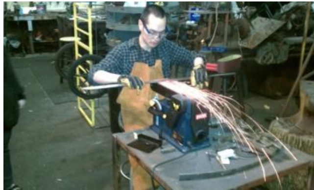
Figure 36: Grinding the Sword.
