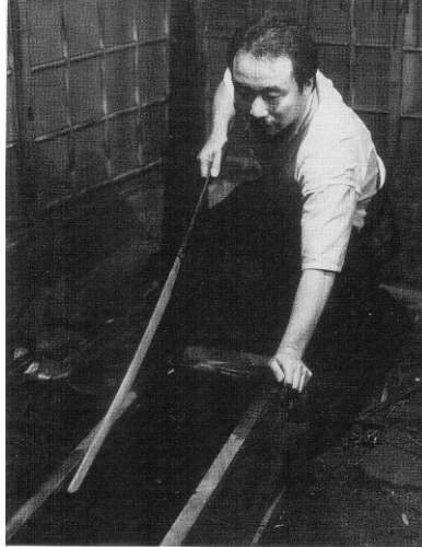
Figure 12: Quenching of the Blade in a Trough of Water.
