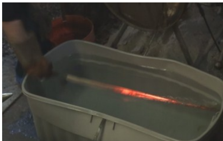
Figure 39: Quenching the Blade.
