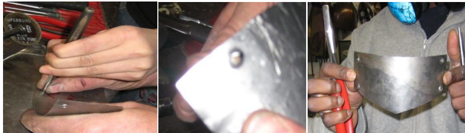
Figure 77. Hole-making with a nail puncher.
