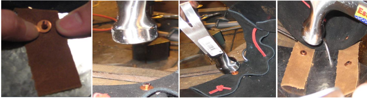
Figure 89. Riveting of the shoulder guards and chest plate.
