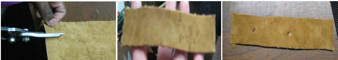
Figure 88. Cutting and punching of holes in the leather strips.
