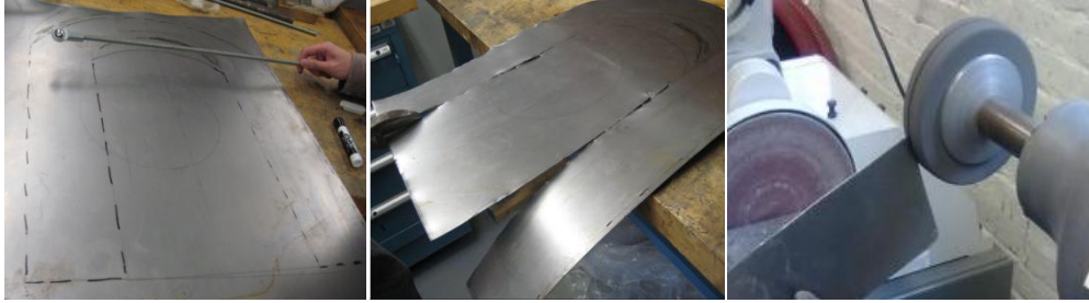
Figure 81. Filing of sharp and rough edges of metal piece.
