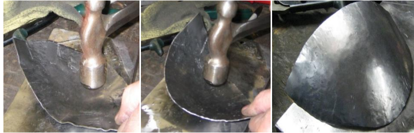
Figure 76. Hammering middle part of Part B.
