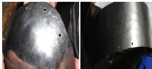
Figure 85. Holes made in shoulder guards and the chest plate.
