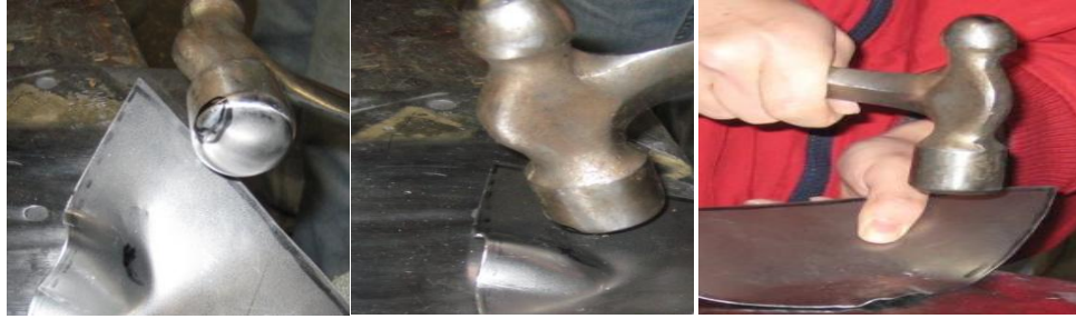
Figure 73. Steps in flattening of the tucks.
