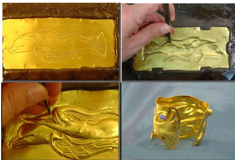
Figure 4. Repousse and chasing of a bracelet. From left to right: Step 1, Step 2, Step 3, and the final bracelet. iv
