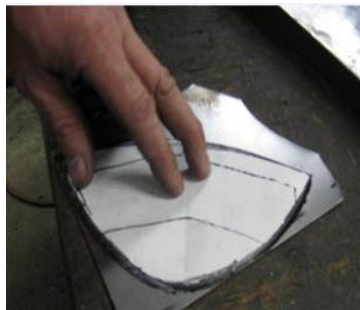
Figure 62. Tracing of shoulder components on metal sheet.
