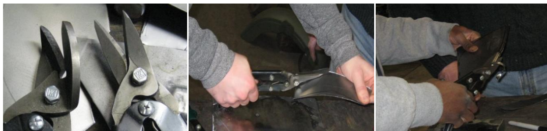
Figure 63. Cutting of metal pieces with shears.
