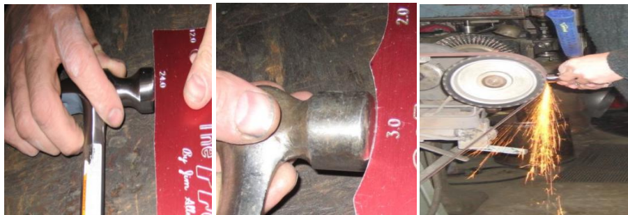
Figure 67. Changing of hammer head radius.
